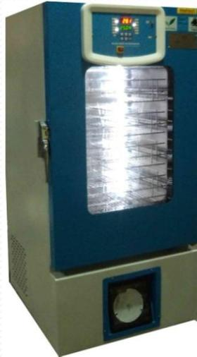
Designed to conform to AABB criteria, the series ensures stable and reliable temperature control utilizing Meditech original technology. A special highly efficient compressor designed and used by Meditech provides rapid cooling and quiet performance for each model.
